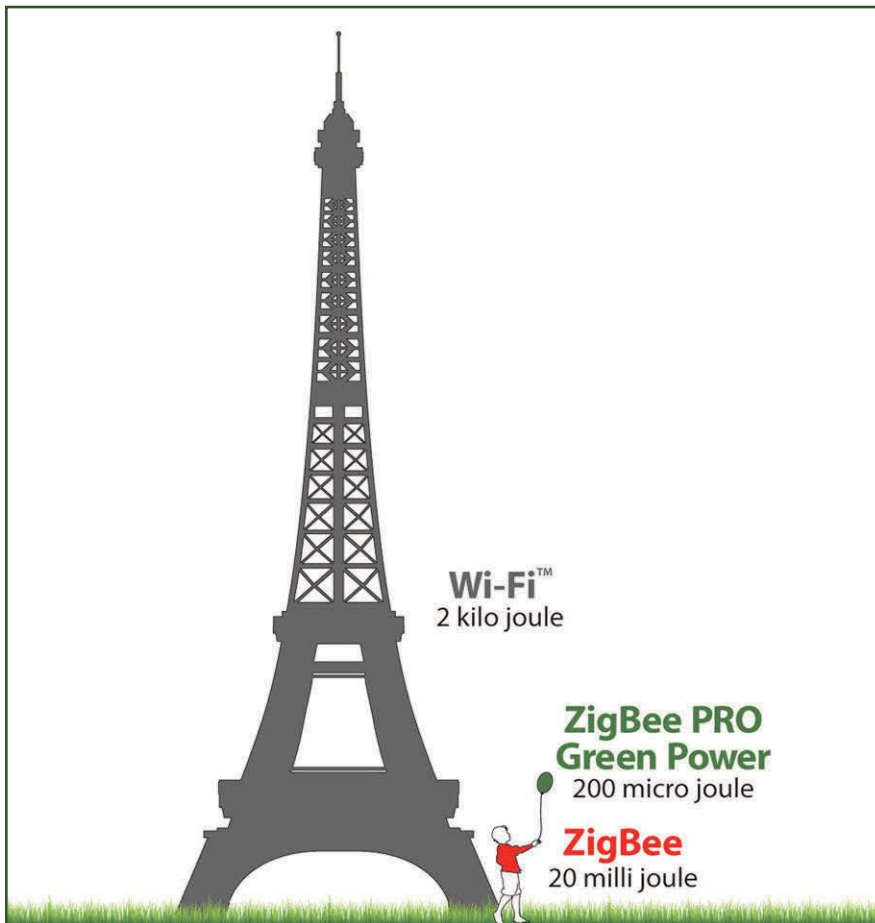
Figure 2 | The ZigBee Green Power feature provides an additional order of magnitude of energy savings in ZigBee networks, consuming only 200 micro joules.
